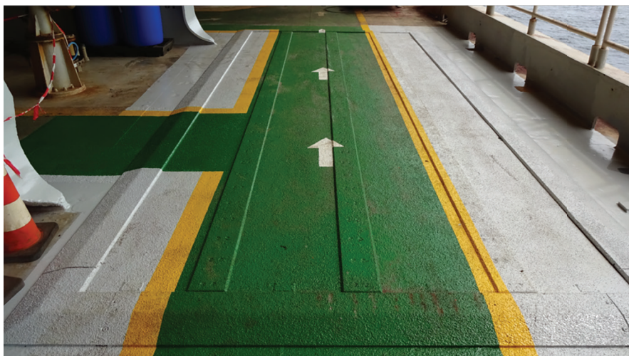
ABOVE: Process-controlled tooling of C-Claw. (All images courtesy Cold Pad) BELOW: Deck repair following application of ColdShield.
