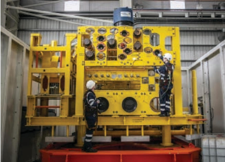
The Subsea CoE in Montrose has the capacity to design, manufacture, and test a complete subsea tree.
