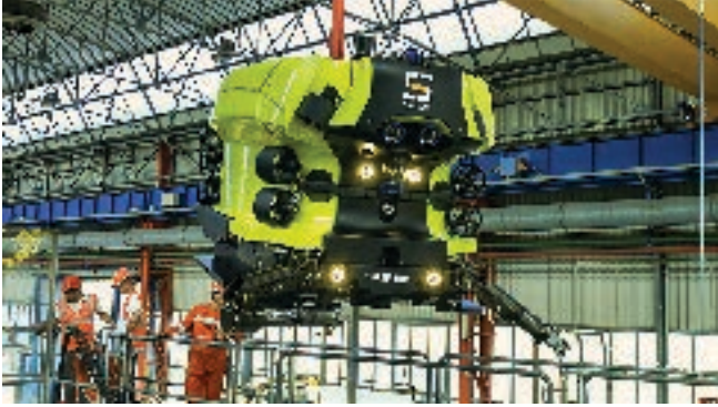
Hydrone-R during tests at Sonsub headquarters in Marghera (Venice).
